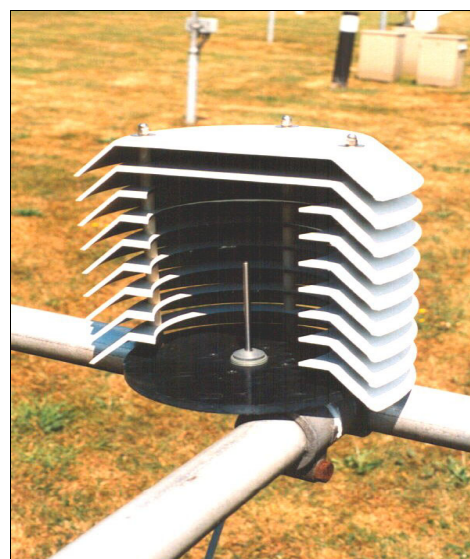
figure 1b: placement of the measuring needle in a cut-away dish screen
