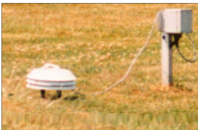
figure 3: dish screen with radiation protection for 10 cm temperature
